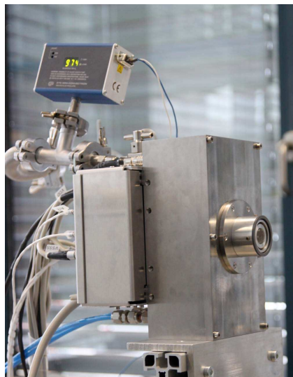
Figure 1: A color X-ray camera has been developed comprising a 48 µm pnCCD for fast X-ray imaging with good spectroscopic performance and subpixel spatial resolution.
