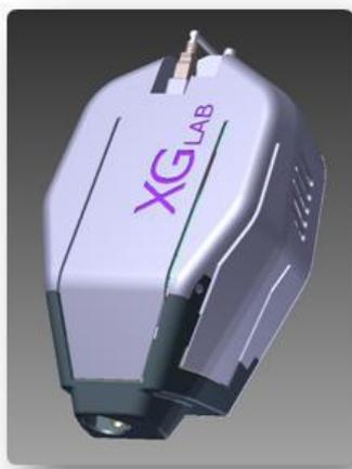
Fig.1. The compact detection head with inside the complete X-Ray SDD detection unit, X-Ray Tube, service sensors. Overall dimension 250x167x110mm, weight <2kg. The unit can operate simply with power connection (12V DC) and a PC with USB2 or Bluetooth connection.
