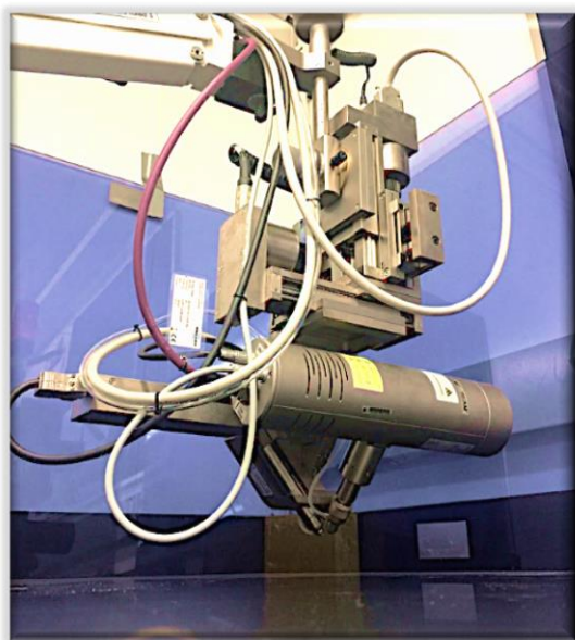
Figure 1. Bruker ARTAX sensor head showing XYZ stages, X-ray tube enclosure, polycapillary optic, fiducial laser, SDD detector and plumbing for He gas flow.
