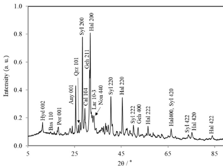
Fig. 1 Identification of crystalline phases in MSWI fly ash.
