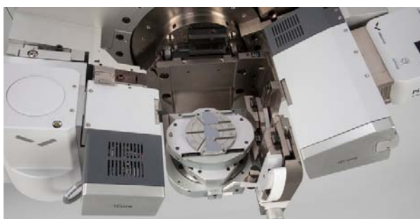
Figure 1 Empyrean configuration with iCore, dCore and Chi-phi-x-y-z sample stage. Multiple samples can be mounted for automated measurements
