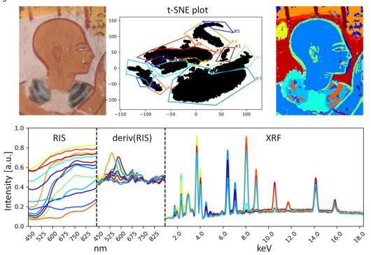
Evaluation of fused XRF and RIS data by t-SNE of a 19<sup>th</sup> dynasty wall painting from the Theban Necropolis, Egypt. The top row shows a visible light photograph, the t-SNE plot with manually selected clusters and the rule/cluster image. In the bottom row average cluster spectra are shown. Adapted from [1].
