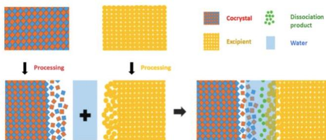
Schematic representation of the impact of lattice disorder on the water mediated dissociation of cocrystals.
