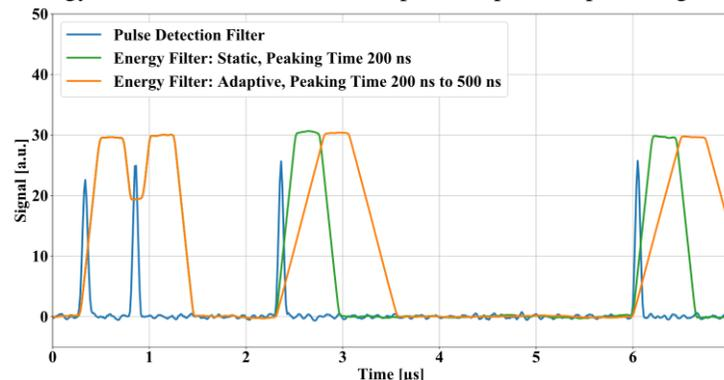
Figure 1: Signal processing with static and adaptive energy filter
