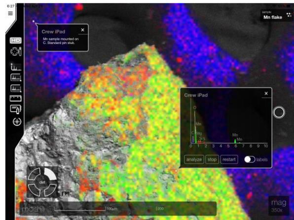
**Figure 2.** EDS spectrum image and point spectroscopy of a Mn flake. Mg and S impurities are detected in the bulk, fine Si particles are on the C background. Bulk Mn signal is mainly from right face of flake due to detector shadowing.
