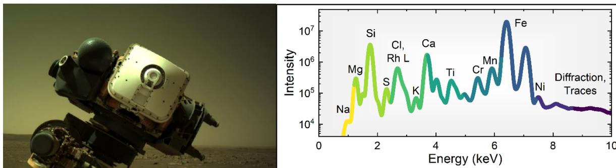
**Figures:** (left) Rover Mastcam-Z image of PIXL sensor head and (right), PIXL spectrum recorded from Dourbes target on sol 257 of the Mars 2020 mission with major element peak labels indicated within.
