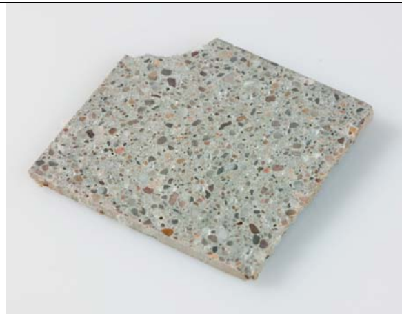
Macroscopic view of the concrete sample 4 x 4 x 0.2cm
