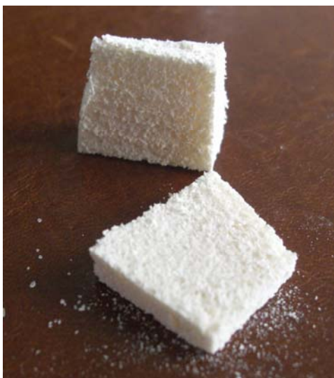
Figure 1: PBX-sample as measured. Cut surface about 1 cm x 1 cm.
