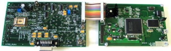
Figure 1 Picture of the complete fast system for multi-channel applications based on SDDs. The left board hosts the 8-channel ASIC, the right board is the fast-DAQ
